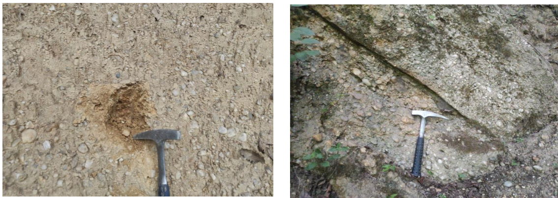
Figure 17. Conglomerate lithology of the trench body km 1+180 (top and bot)
